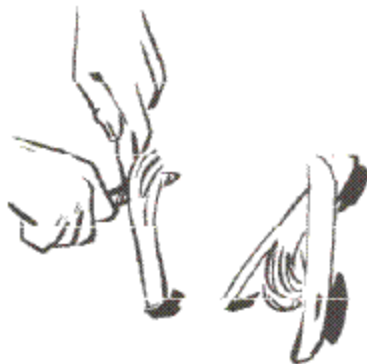
The fuzzi-stick fire starter is made by whittling a dead stick, leaving all of the shivers attached.
